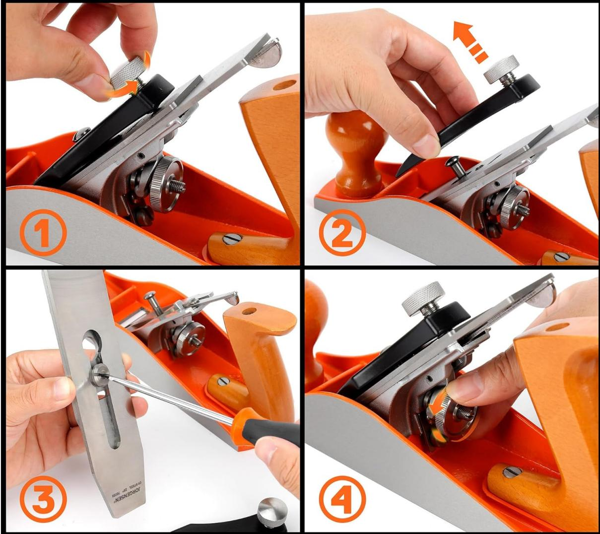
This image provides a step-by-step guide for replacing the planer blade. Step 1 shows loosening the clamping mechanism. Step 2 illustrates removing the old blade assembly. Step 3 details attaching the new blade to the chip breaker. Step 4 shows reinserting the assembled blade into the plane body.
