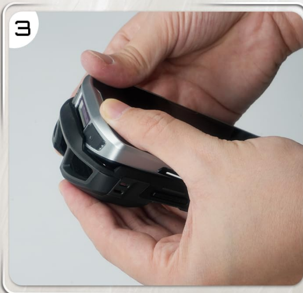
Figure 4: The case supports attachment of optional trigger handles for increased efficiency.
