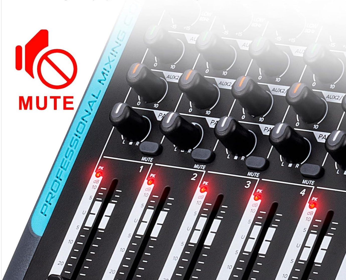
Figure 8: Close-up of the mute buttons and their indicator lights on the DP-10 mixer, allowing individual channel silencing.
