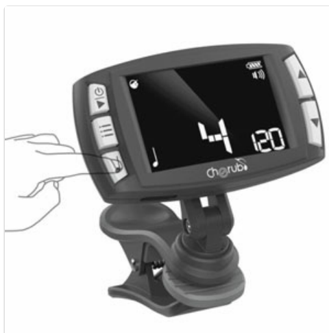
Image 4.2: A hand demonstrating the use of the Item button, which is used for functions like Tap Tempo in Metronome mode.
