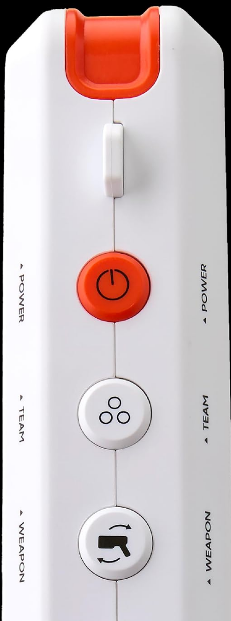
Image: The top of the blaster with clearly labeled Power, Team, and Weapon buttons.
