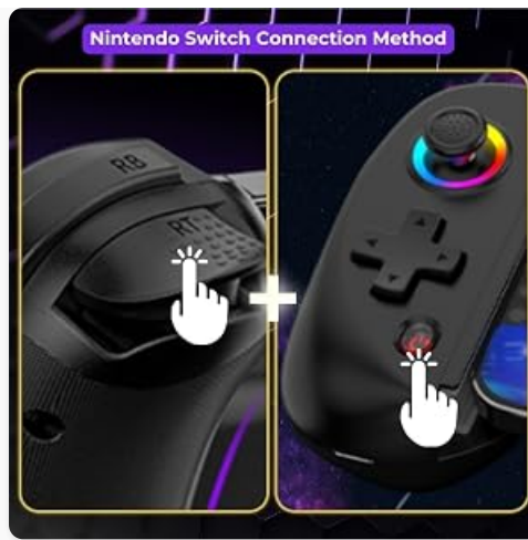
Nintendo Switch Connection Method (RT + Power)
