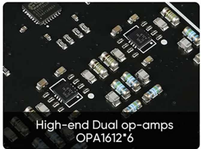
Image: Internal view of the SMSL DO100PRO circuit board, showcasing the built-in low-noise power supplies, the Qualcomm QCC5125 Bluetooth chip, and the high-end dual op-amps OPA1612.
