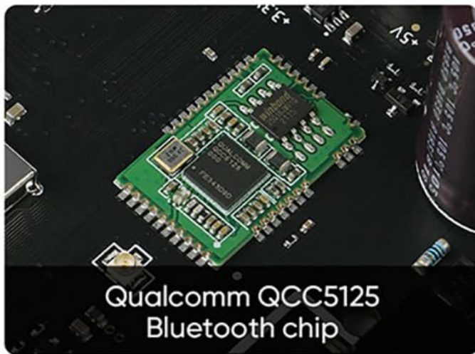
Image: Internal view of the SMSL DO100PRO circuit board, showcasing the built-in low-noise power supplies, the Qualcomm QCC5125 Bluetooth chip, and the high-end dual op-amps OPA1612.
