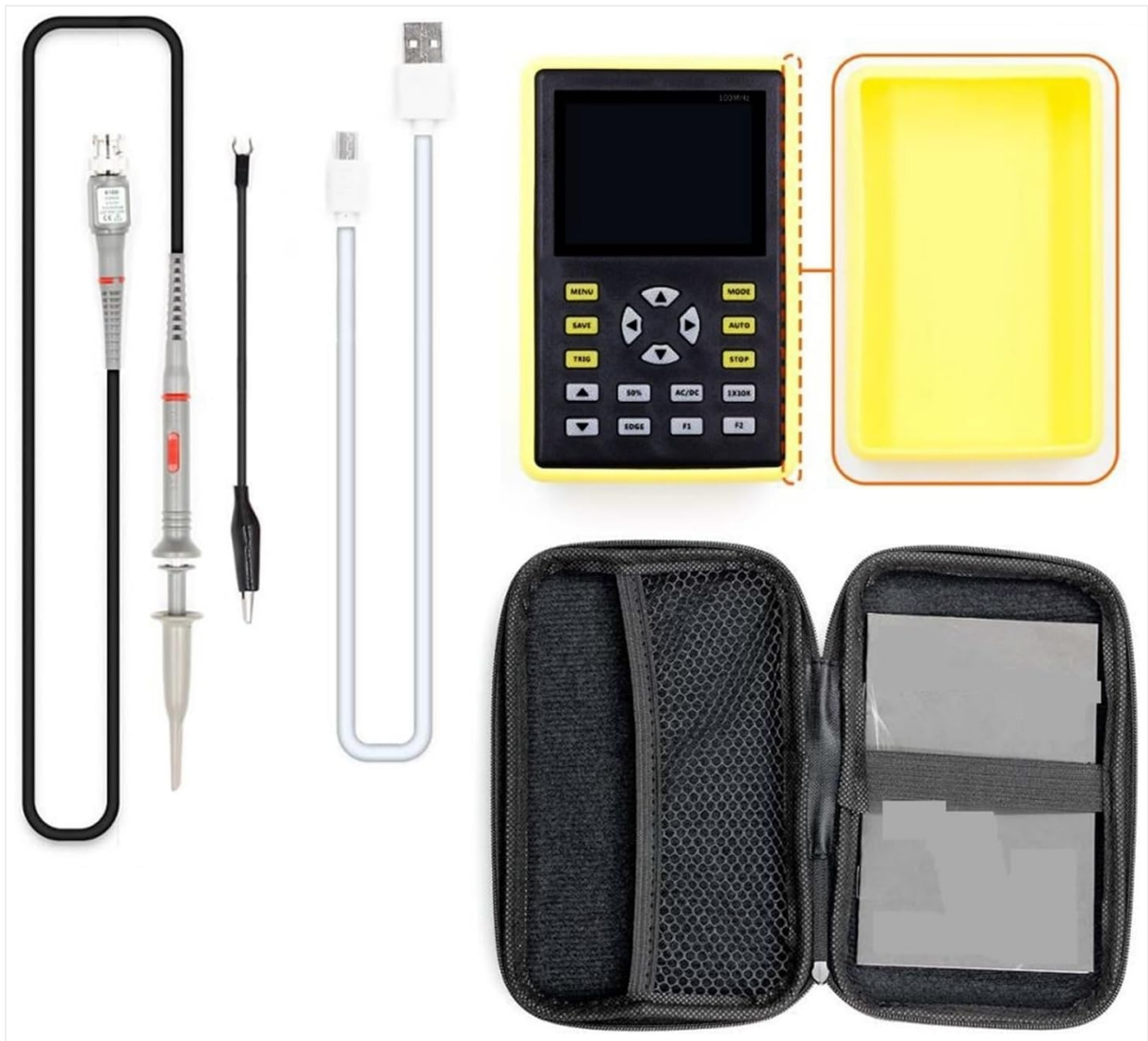
Figure 2.2.1: The ZHDBD 5012H Digital Oscilloscope package includes the main unit, a probe, a USB cable for charging and data transfer, and a protective carrying case.
