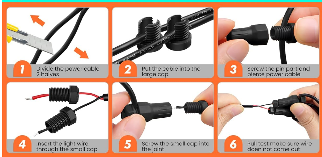
Image: Step-by-step guide for connecting the low voltage wires to the landscape lights using the provided connectors. Note: Low voltage wires and transformer are not included.
