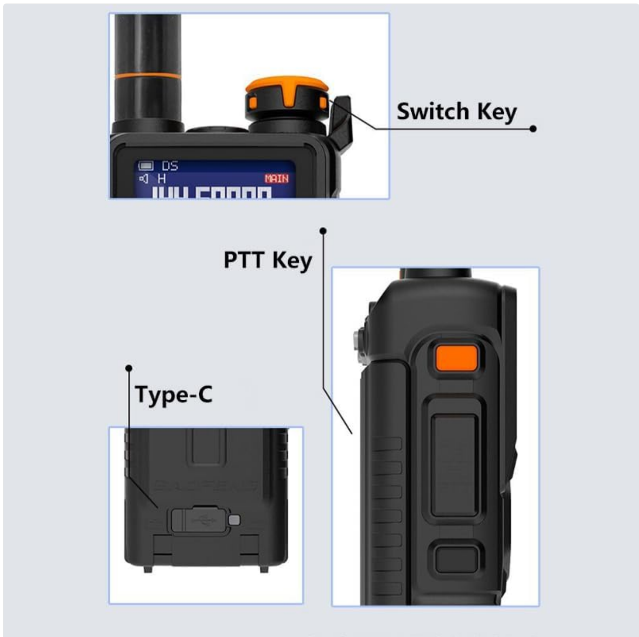
Image 3.2: Detailed view of the BAOFENG K5 Plus radio, indicating the location of the power/switch key, Push-to-Talk (PTT) button, and the Type-C USB charging port.
