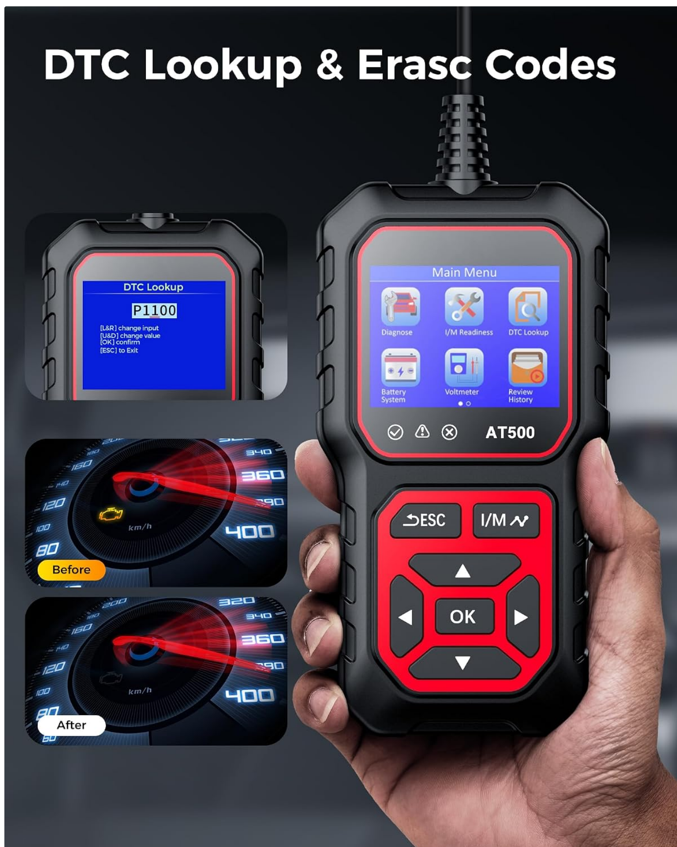
Image: The GEARELEC AT500 displaying a DTC lookup result (P1100) and illustrating the effect of clearing a check engine light, showing a dashboard before and after the light is extinguished.
