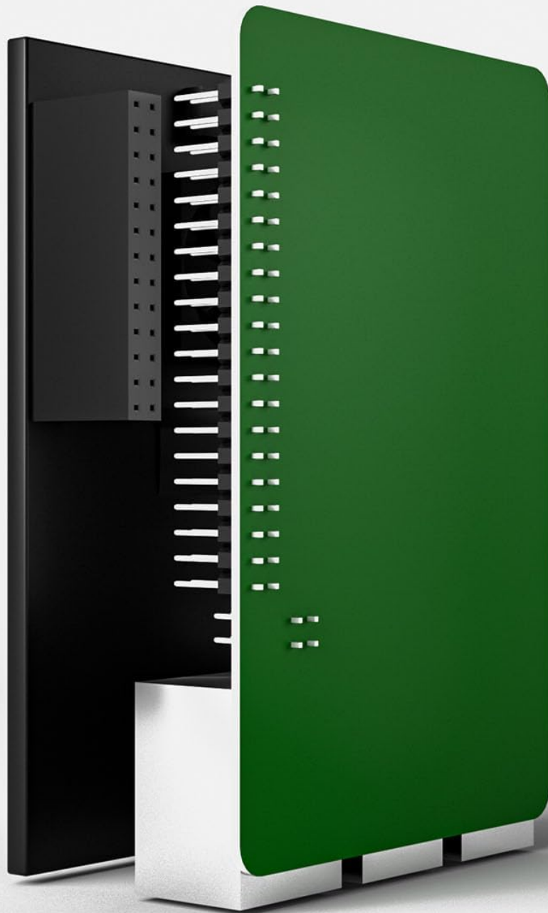
Image 3.2: Detailed view of the SPI interface, emphasizing the correct pin alignment for connection to avoid damage.
