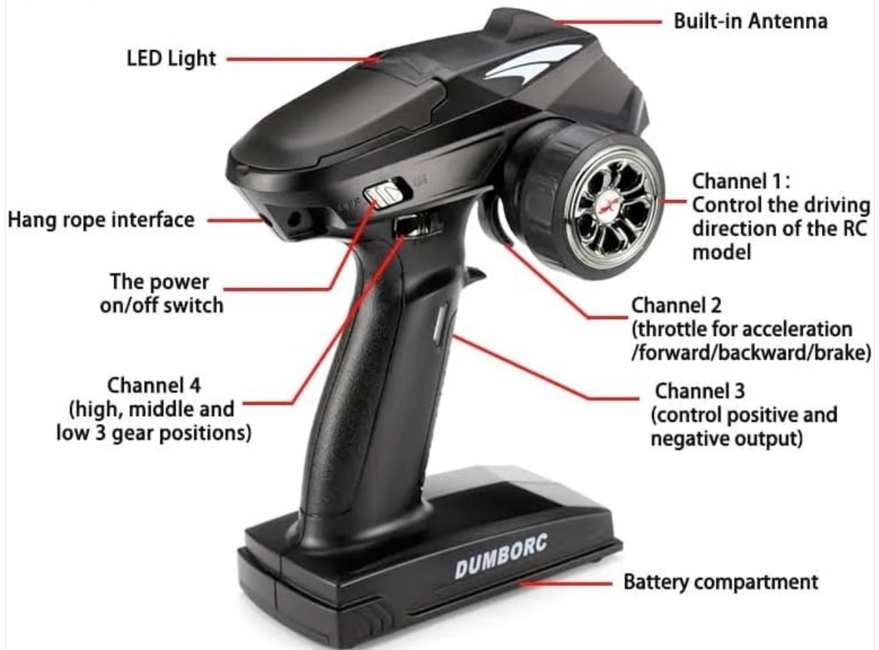
Figure 2: Detailed view of the DUMBORC X4 Transmitter's channel functions and components.
