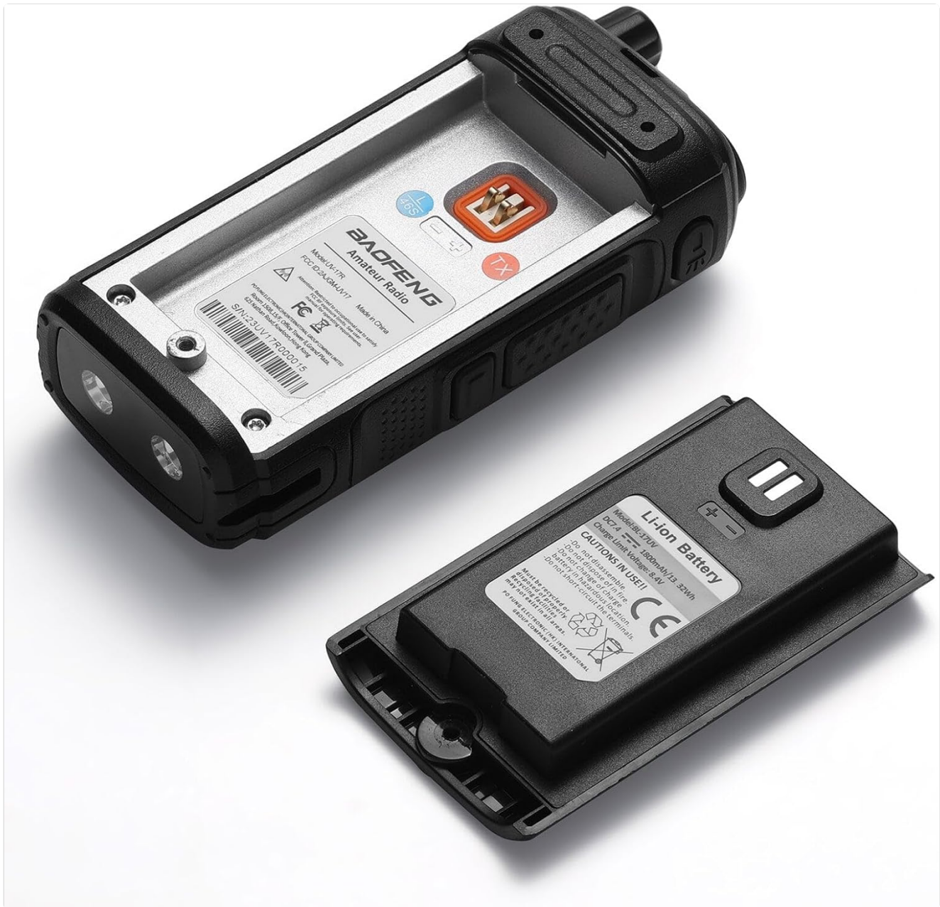
Figure 3: Battery installation process for the UV-17R.
