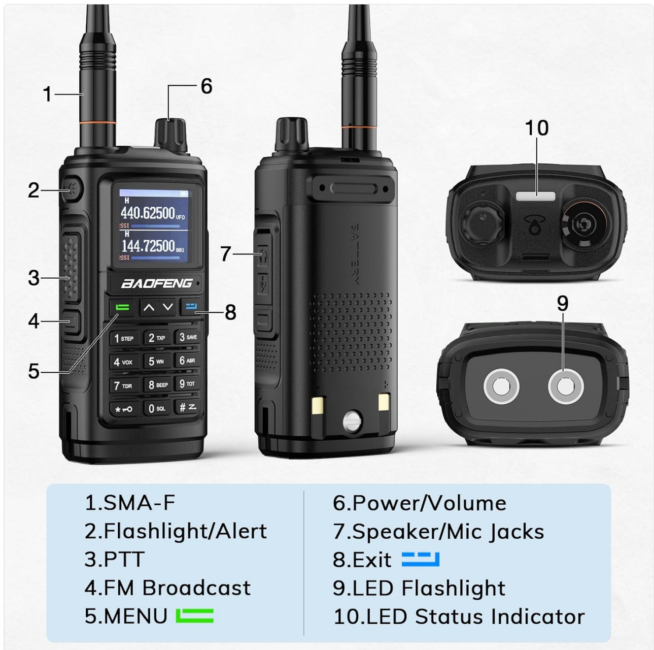
Figure 4: Key components and controls of the UV-17R.
