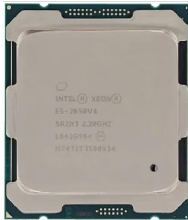
Image: A close-up top view of the Intel Xeon E5-2650 V4 CPU, showing its integrated heat spreader.
