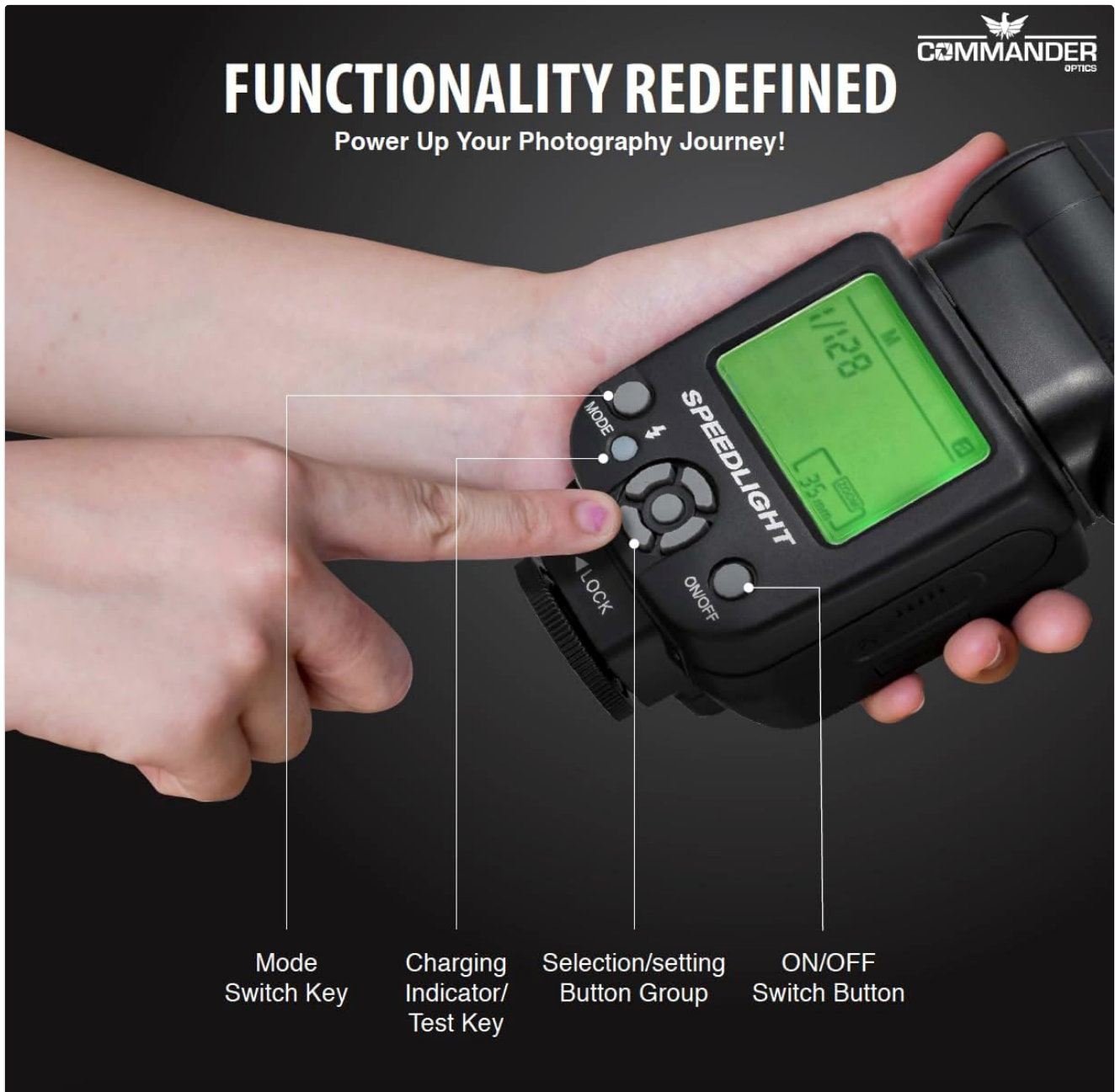
Figure 4.1: Front view of the Speedlite flash with control labels.
