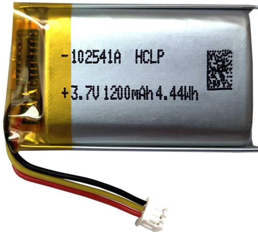
Image 1.1: XINLANTECH 1200mAh Lithium Polymer battery, designed for Sena Spider ST1 Motorcycle Bluetooth Communication System. The battery features a white connector and three colored wires (red, black, yellow).
