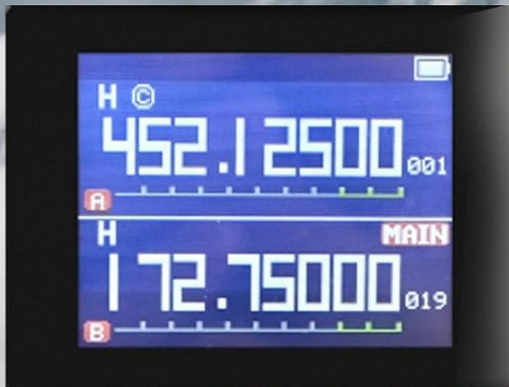
Image: Multi-band frequency ranges and the 1.77-inch TFT screen display.
