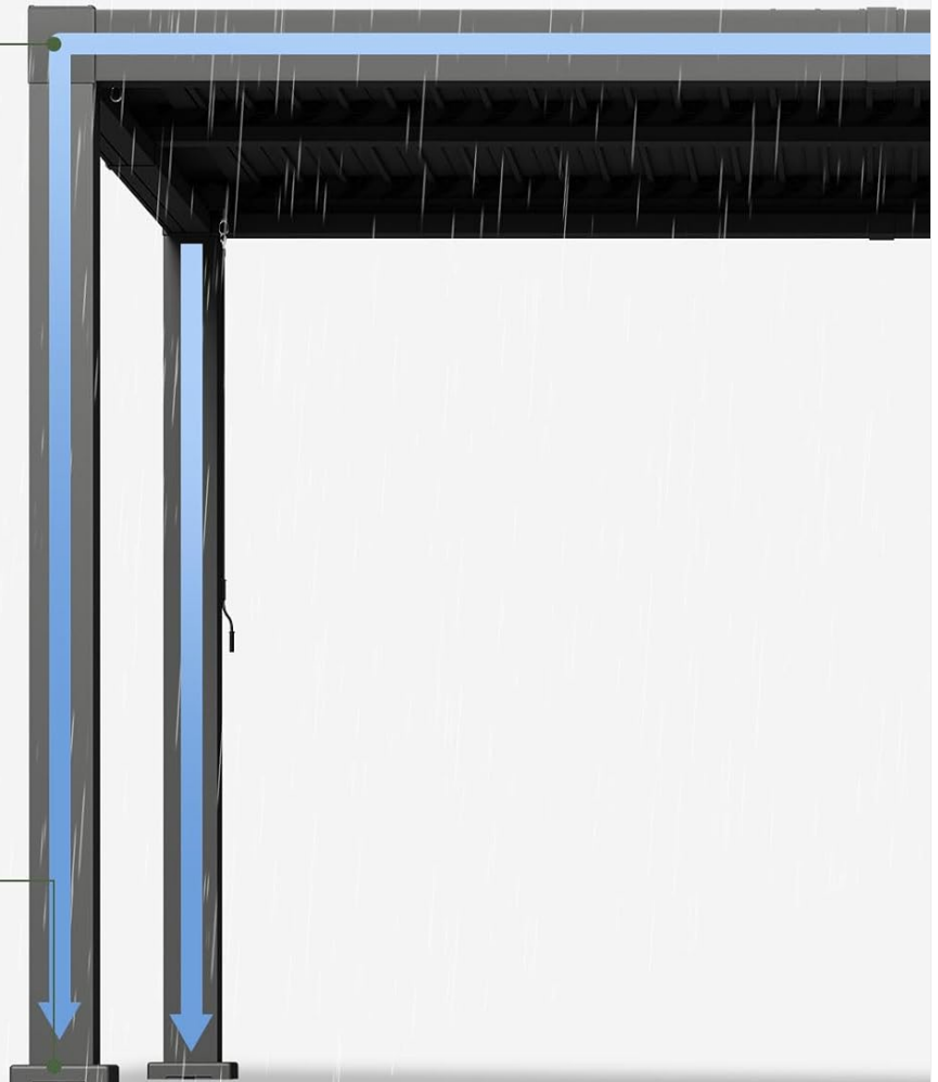
Figure 7: Integrated Drainage System
