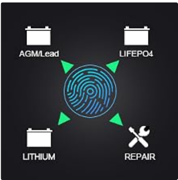
Figure 5.2: Battery type selection interface, allowing choice between AGM/Lead, LiFePO4, Lithium, and Repair modes.
