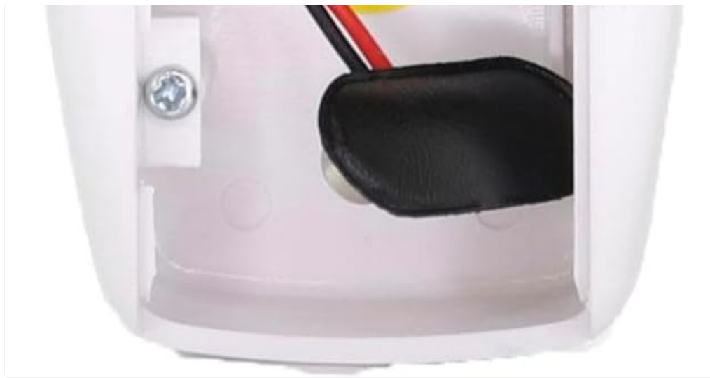
Image: Back view of the Anderic RR7070T remote control with the battery compartment open, showing where to insert the 9V battery.
