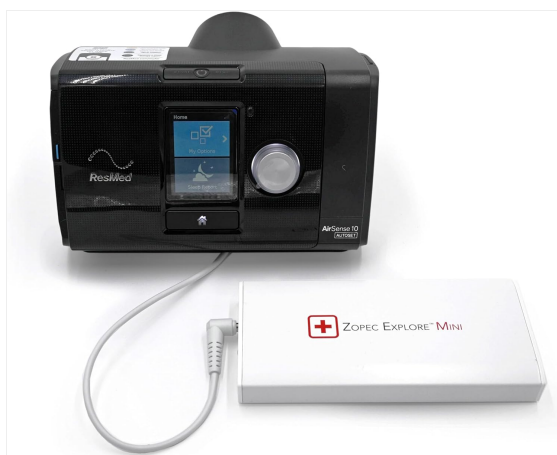
Figure 5: Connection with ResMed AirSense 10.
