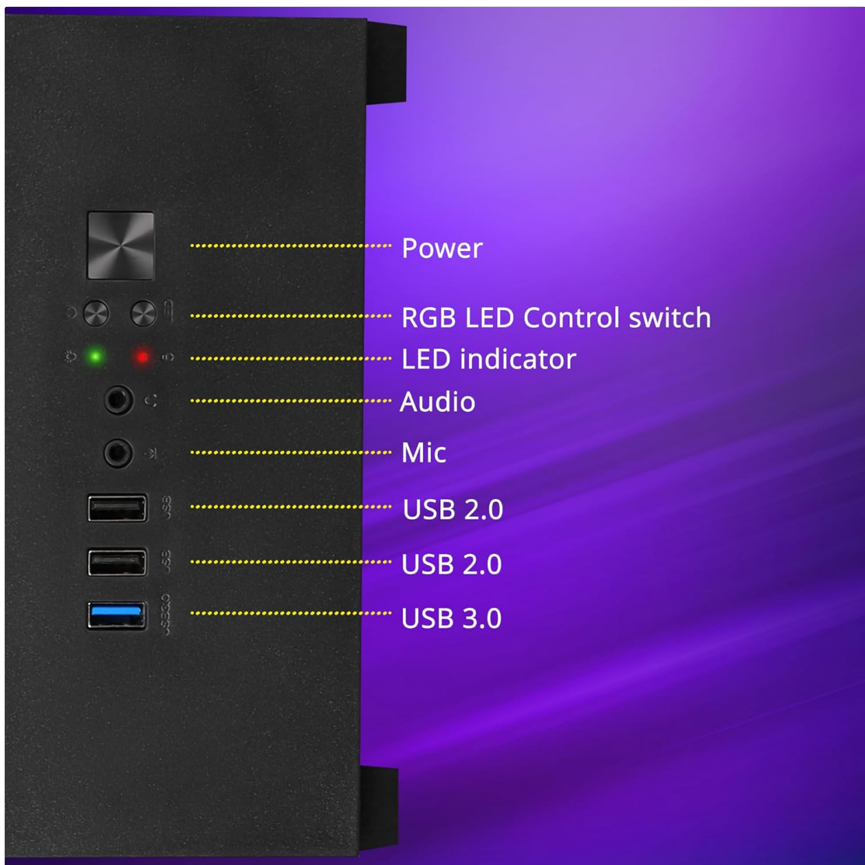
Image 2.2: Detailed view of the front panel I/O, showing the power button, RGB LED control switch, LED indicators, audio ports, and USB ports.
