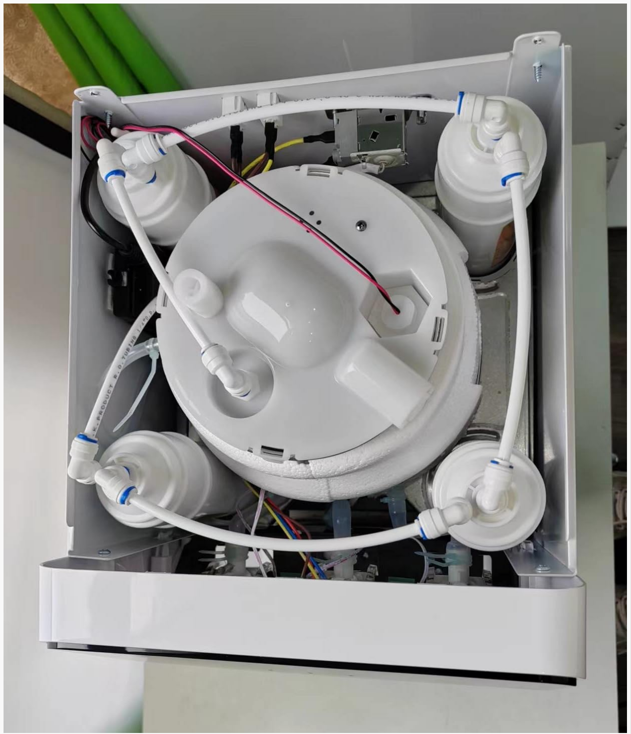
Image 5.2: Internal view showing the 4-stage filtration system and water tubing.
