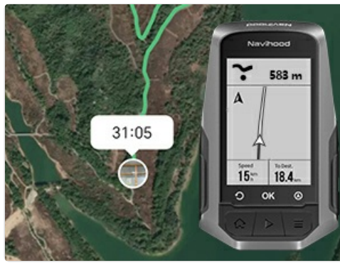
Image: The MEILAN Navihood L1 displaying a route deviation warning, indicating that the user is off course and providing a visual cue to return to the planned route.
