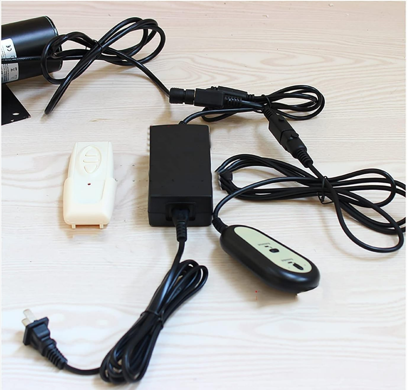
Image 5: Components for controlling the motorized TV mount, including the wireless remote control, the wired switch, and the power adapter.
