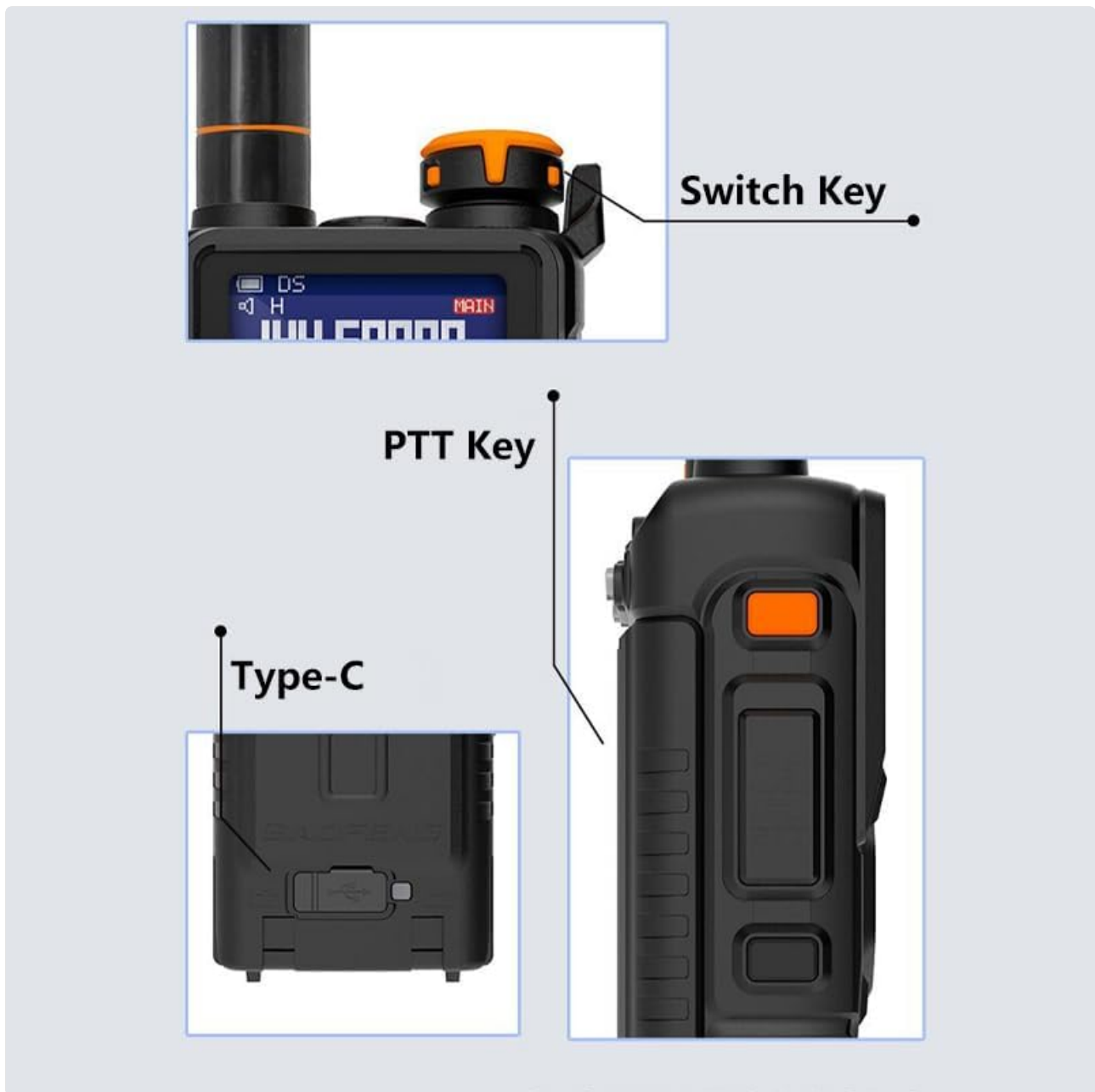
Figure 2: Key physical features of the BAOFENG K5 Plus, including the power/switch key, Push-to-Talk (PTT) button, and USB Type-C charging port.
