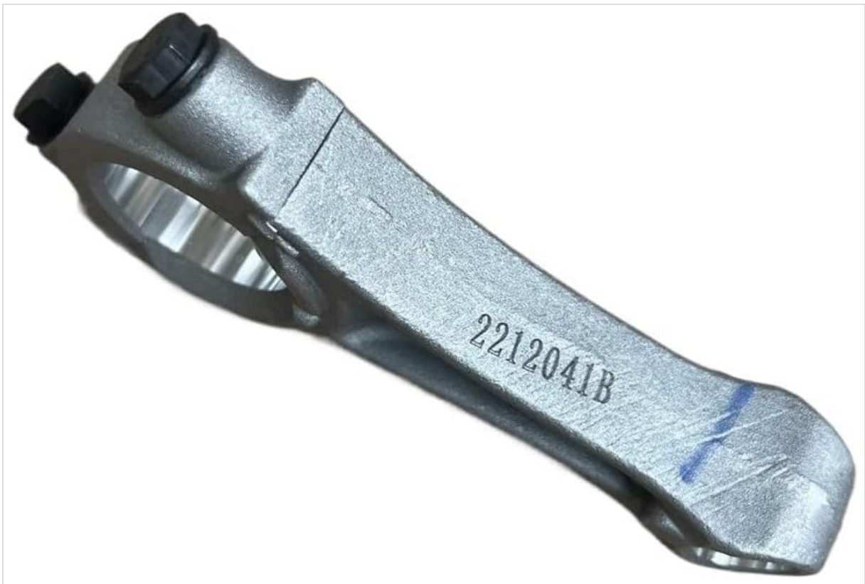
Figure 2.3: Side view of the ROEDE Connecting Rod, showing the stamped part number '2212041B' for identification.
