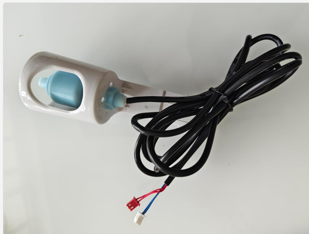
Figure 5: The water float switch, which detects the water level in the ice maker's reservoir.
