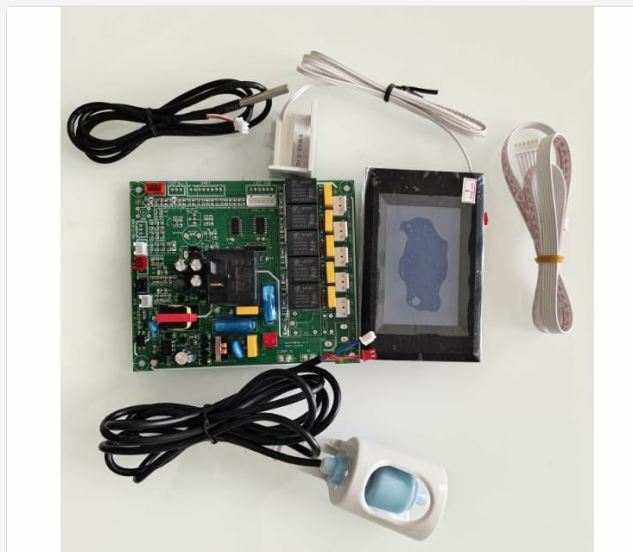
Figure 1: Complete Ice Maker Control Board Kit, including main board, touch screen display, and various sensors.
