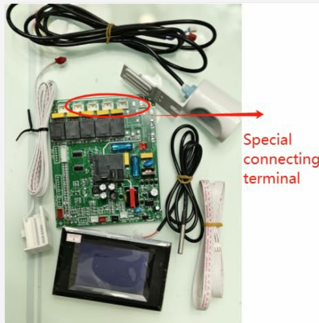
Figure 2: All components of the control kit, highlighting the special connecting terminal on the main board.
