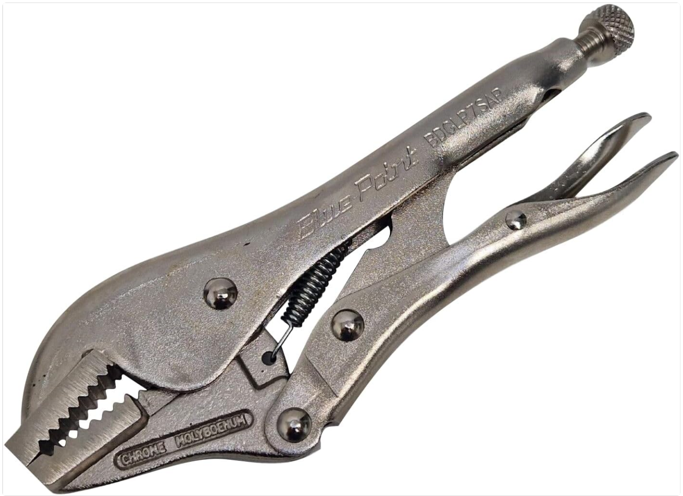
Figure 2: The 7-inch Straight Jaw Locking Pliers, designed for secure gripping of flat, square, or hex materials. These pliers are engineered to provide maximum contact on flat, square, or hex workpieces. The hardened teeth are designed to grip from any angle, ensuring a secure hold. The adjusting screw allows for precise pressure control, and the guarded release trigger protects against accidental release.
