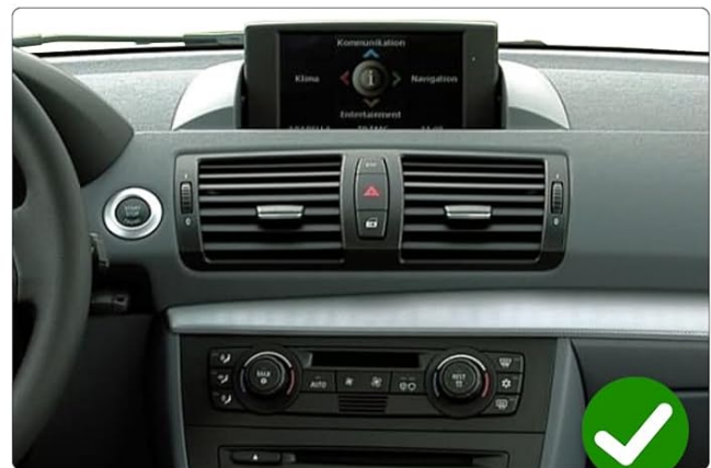
Image 2.1: Visual guide for identifying compatible CCC system and incompatible NBT/CIC systems.
