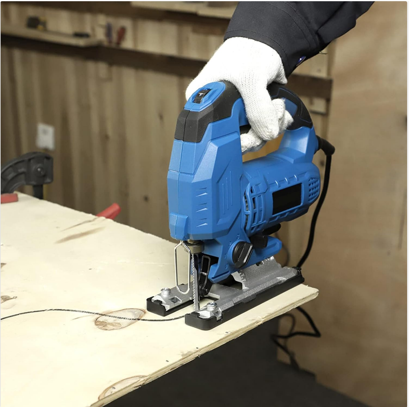
Figure 6: A user demonstrating the proper grip and operation of the jigsaw while cutting wood.
