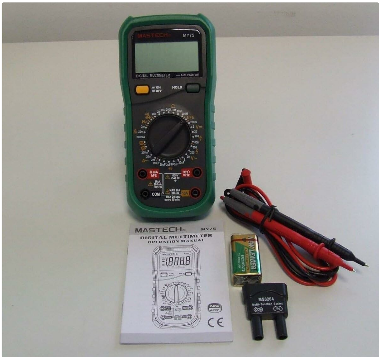
Figure 3.2: The MASTECH MY75 Multimeter with its essential accessories: test leads, LR44 batteries, and the multi-function hFE socket.
