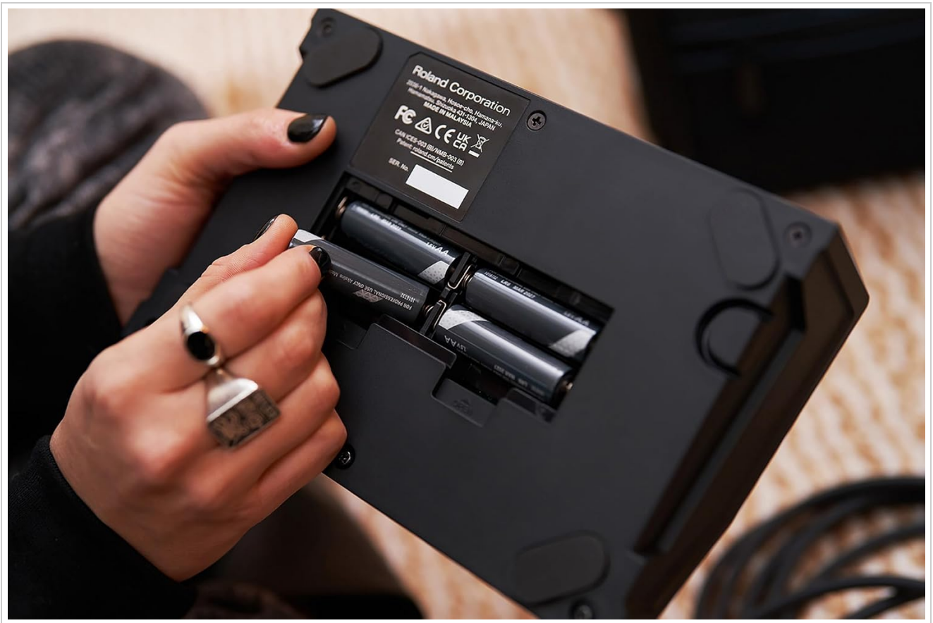
Image: A user installing four AA batteries into the battery compartment located on the underside of the BOSS VE-22 pedal.
