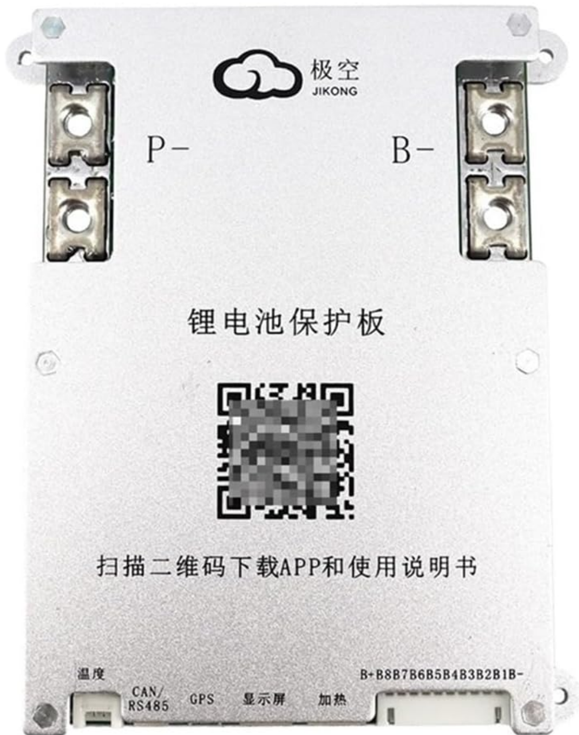
Image: Front view of the JK Smart BMS B1A8S10P, showing the main terminals and QR code for app download.
