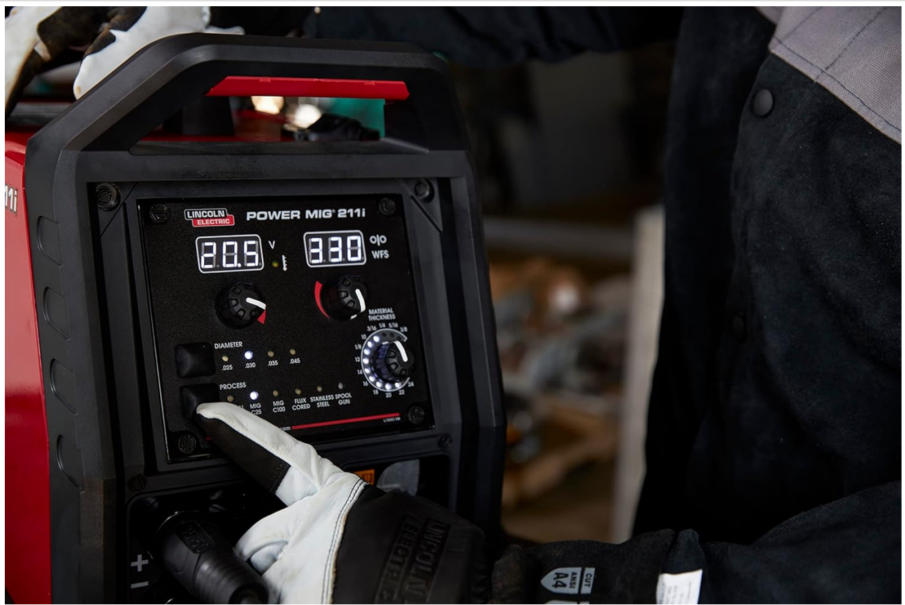
Figure 4.1: Control panel for process, diameter, and material thickness selection.
