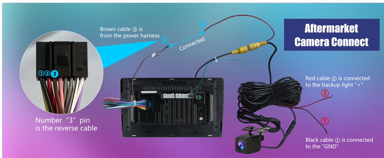
Image: A visual guide demonstrating how to connect an aftermarket reverse camera to the car radio system, detailing the connections for ground, backup light positive, and the reverse cable from the power harness.
