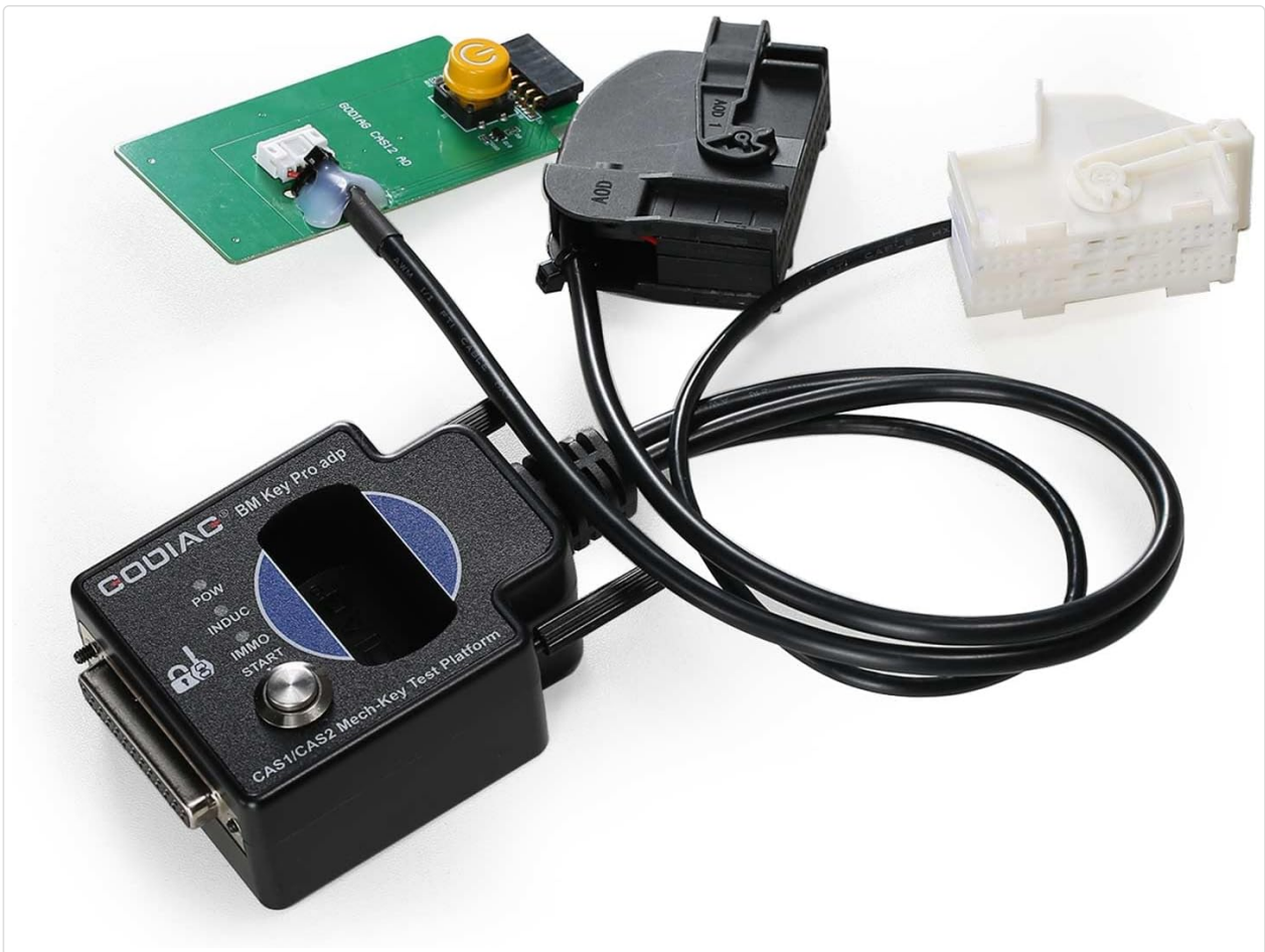
Figure 4.4: An annotated diagram highlighting the various parts of the GODIAG CAS1/CAS2 Test Platform, including indicator lights (Power, IMMO, INDUC), key identification port, start switch, and connectors for CAS1 (54PIN) and CAS2 (41PIN, 14PIN) modules, along with the start/stop button.
