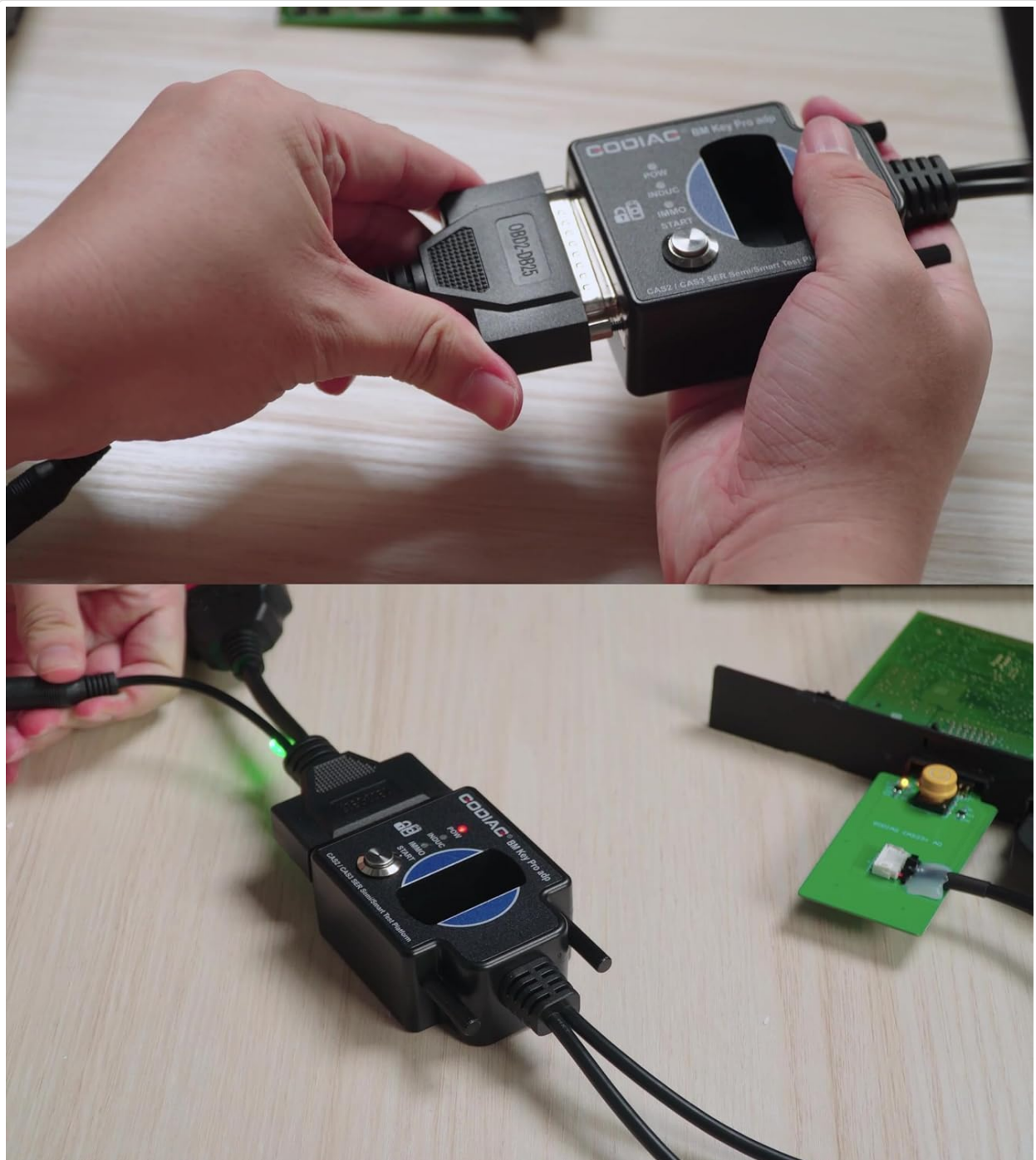
Figure 4.1: A close-up view of hands connecting the OBD2-DB25 cable to the main GODIAG test platform unit, illustrating the secure attachment of the primary data cable.
