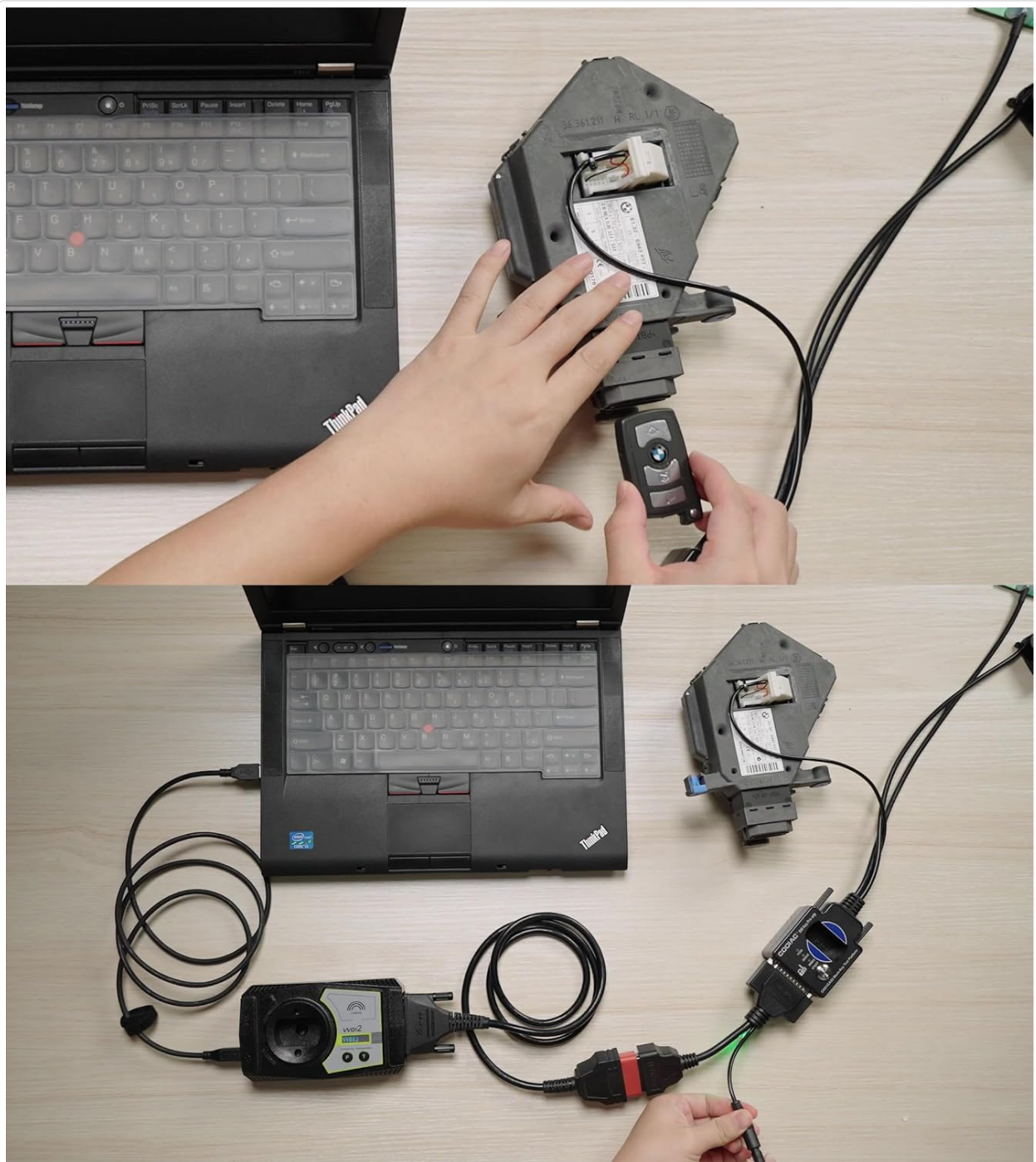
Figure 4.2: This image shows the connection of the power supply cable and the OBD2 diagnostic cable to the GODIAG test platform, indicating readiness for operation.
