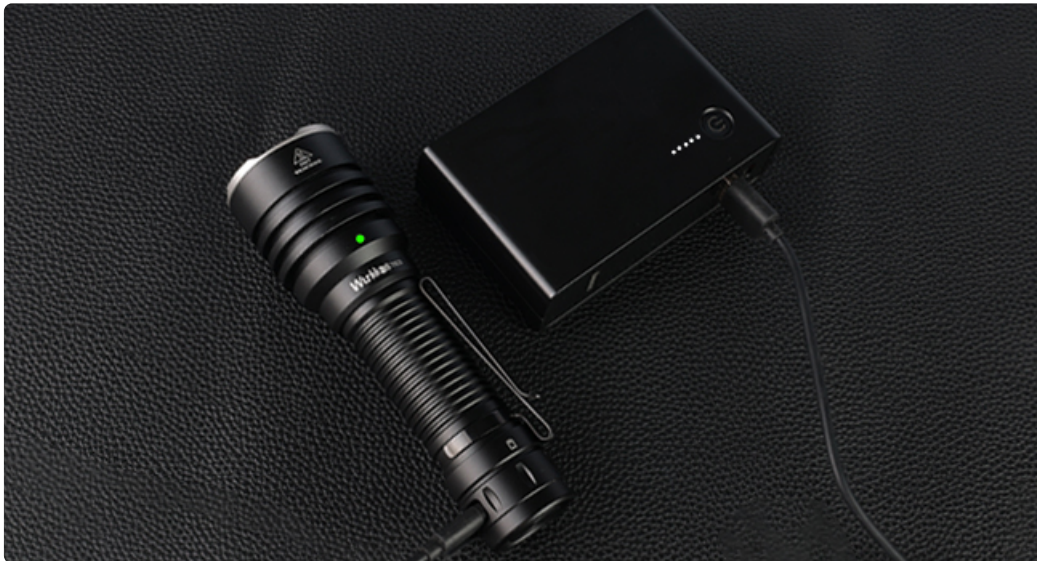
Figure 4.1: Charging the TS23 via its USB Type-C port.
