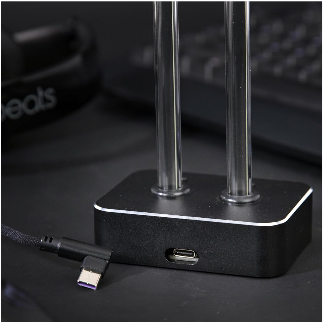
Image 3.3: Rear view showing the USB Type-C power input port.
