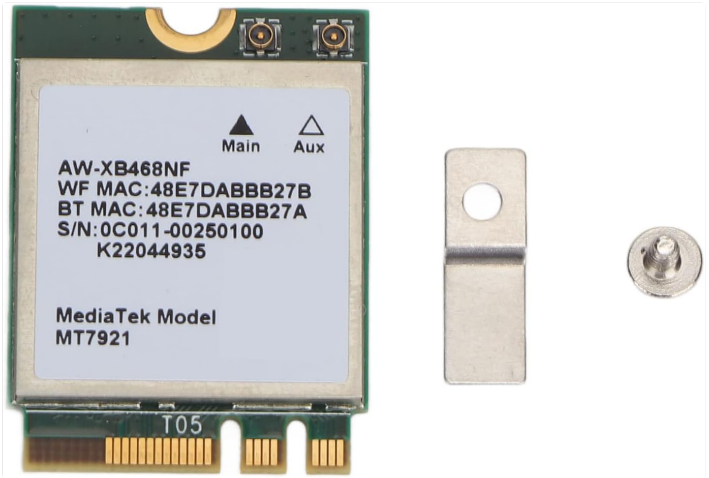
Image 3.1: The network card along with the included gasket and screw for installation.
