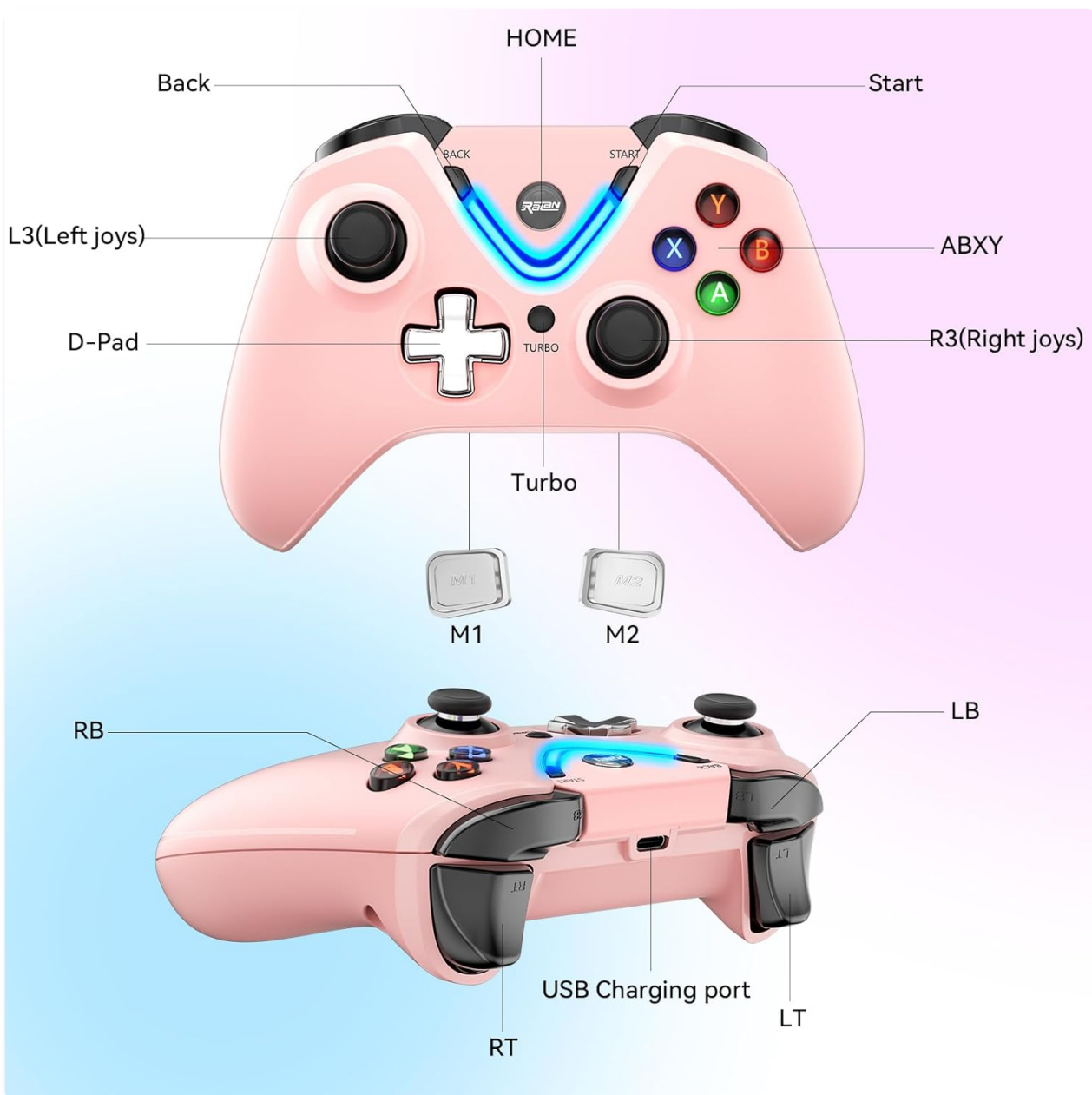
Figure 3.1: Controller Layout - This image displays the RALAN Wireless Controller from a top-down and angled view, with various buttons and ports clearly labeled. Key labels include HOME, Start, Back, L3 (Left joystick), R3 (Right joystick), D-Pad, ABXY buttons, Turbo button, M1/M2 paddles, RB/LB (shoulder buttons), RT/LT (triggers), and the USB Charging port.
