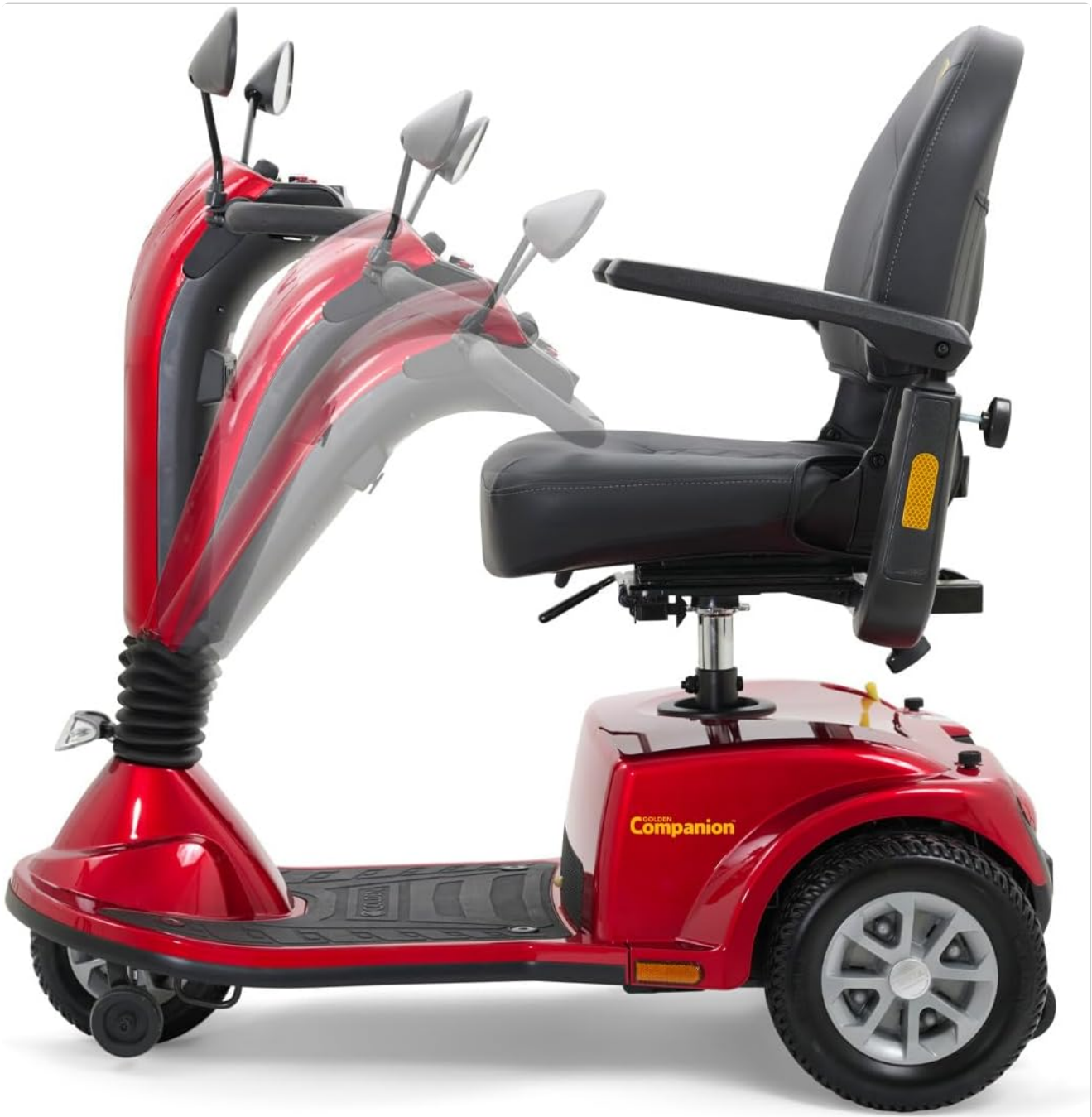
This image demonstrates the adjustable tiller feature of the scooter, showing how it can be positioned for user comfort.
