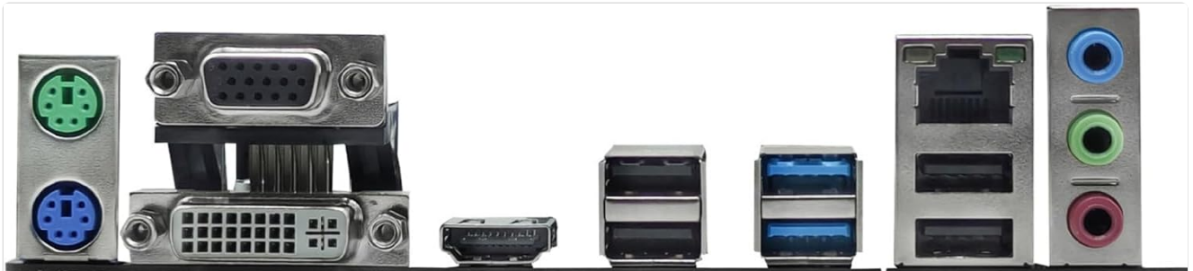
Figure 2: Rear I/O Panel of the Dpofirs H310 Motherboard. From left to right, it displays PS/2 ports, VGA port, DVI port, HDMI port, USB 2.0 ports, USB 3.0 ports, RJ45 LAN port, and audio jacks.
