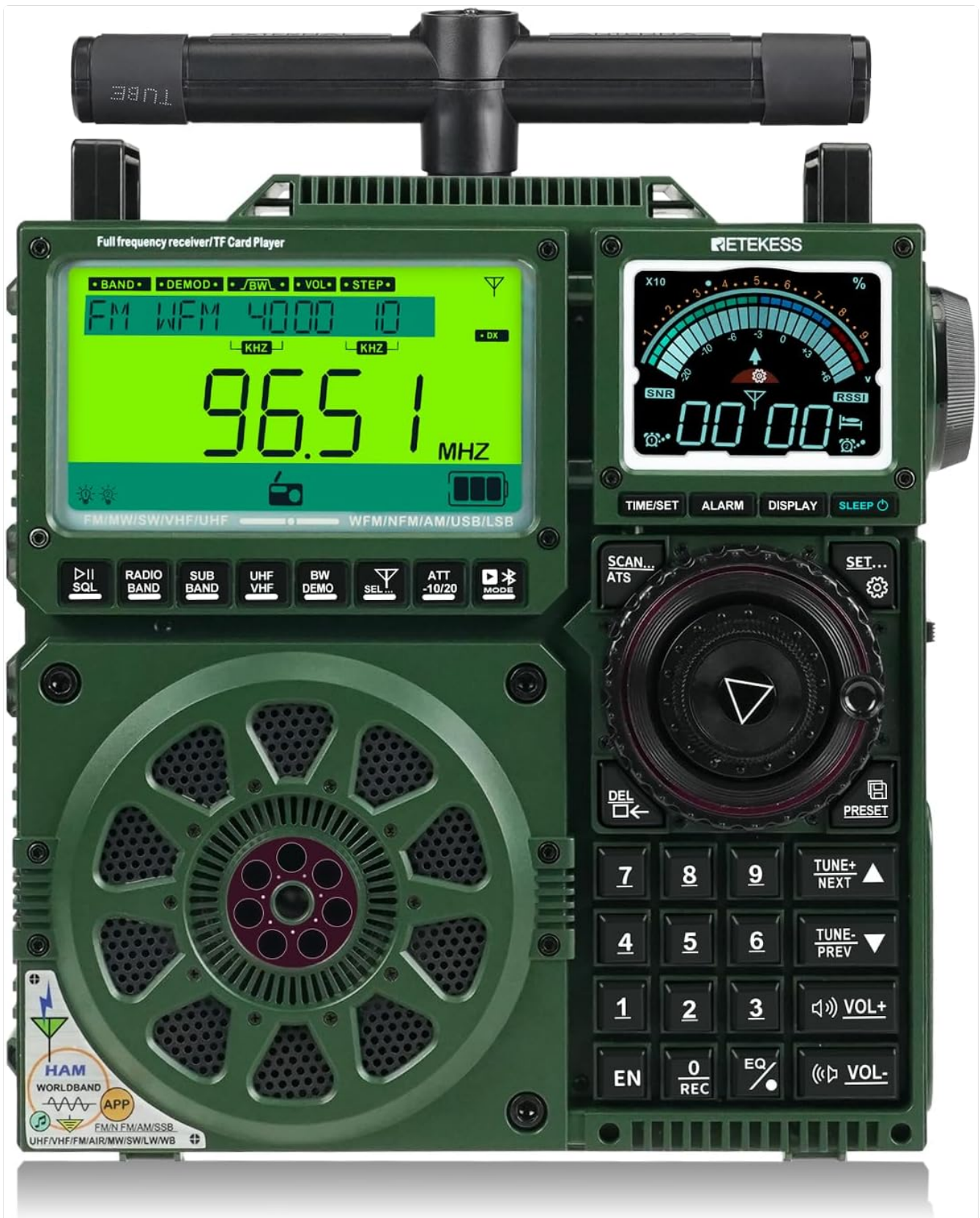
Figure 3.1: Front panel of the TR113, illustrating the main display, secondary display, keypad, and tuning controls.
