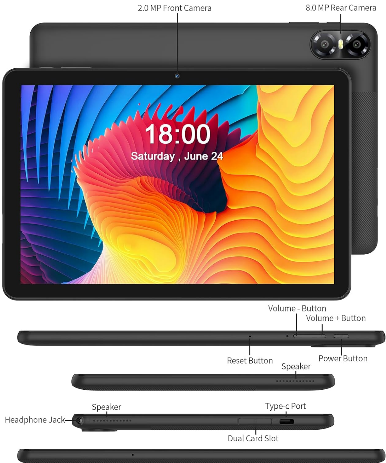
Image 1.2: Hardware overview of the PRITOM M10 Tablet, indicating button and port locations.
