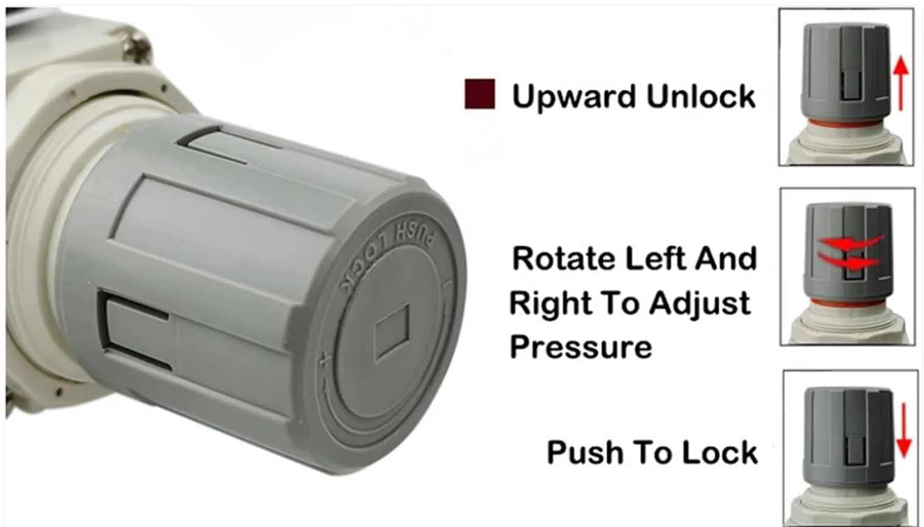
Figure 4: Instructions for adjusting the pressure using the adjustment knob: Upward Unlock, Rotate Left and Right to Adjust Pressure, Push to Lock.
