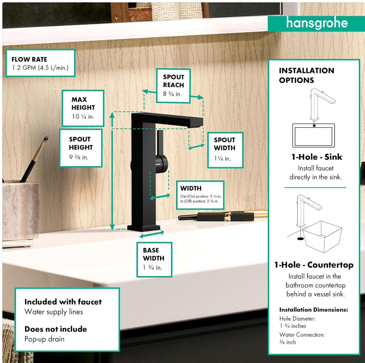
Image: Detailed diagram showing the dimensions of the Hansgrohe Tecturis E faucet, including flow rate (1.2 GPM), max height (10 1/4 in), spout height (9 5/8 in), spout reach (8 3/4 in), spout width (1 1/4 in), width (3 1/4 in on, 2 5/8 in off), and base width (1 3/4 in). Also illustrates 1-hole sink and 1-hole countertop installation options, specifying a hole diameter of 1 3/4 inches and 3/8-inch water connection.
