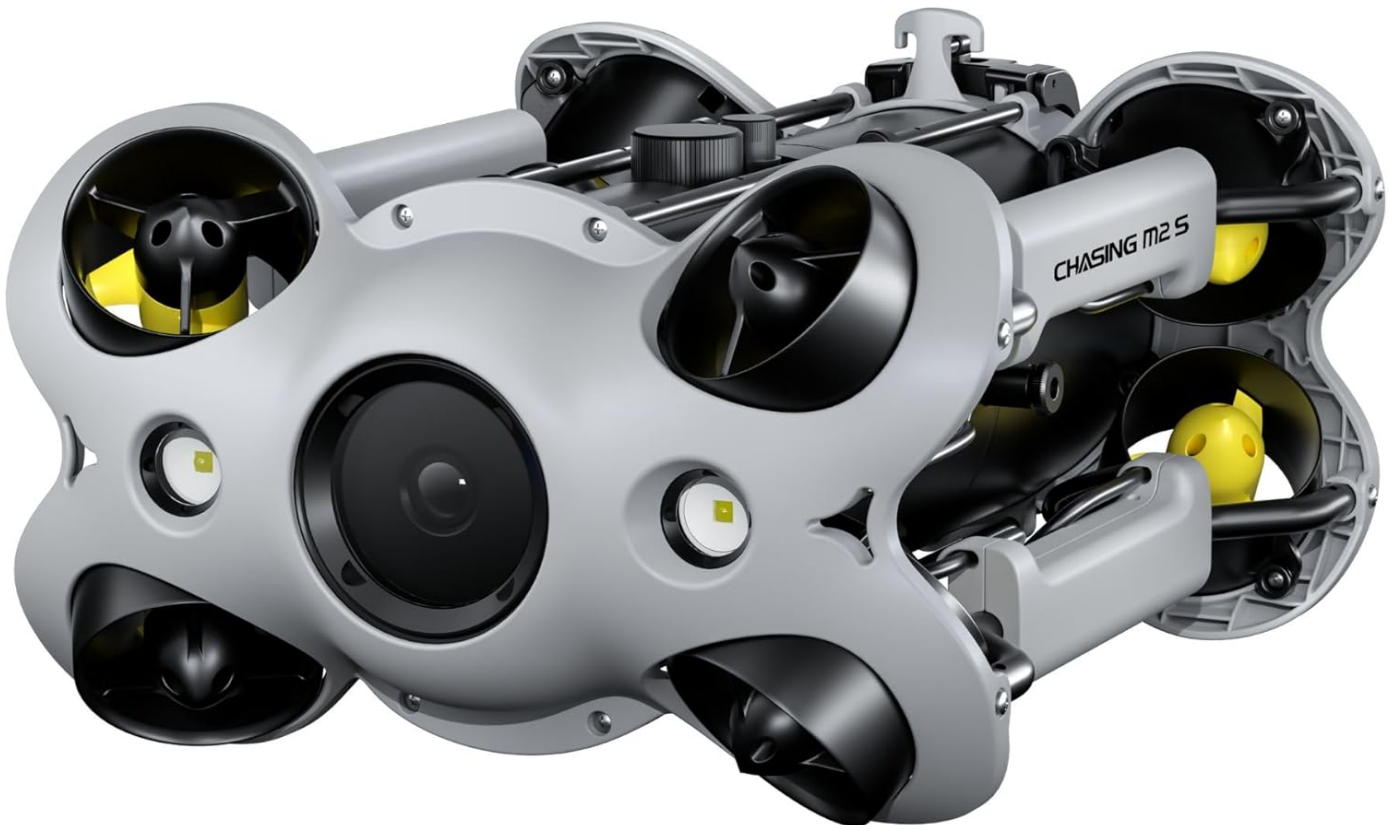
Figure 4.2: Front view of the Chasing M2 S Underwater Drone, showcasing its camera lens and integrated LED lights.
