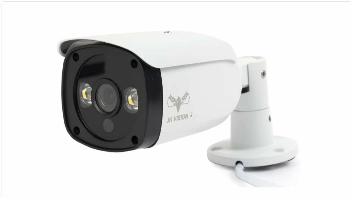
Figure 3.2: A single JK Vision 5MP IP Bullet Camera, featuring a robust housing and integrated lens. These cameras capture crisp, high-resolution 5-megapixel footage. They are designed for both indoor and outdoor use, featuring color night vision and built-in audio capabilities for comprehensive surveillance.
